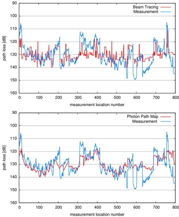
Fig. 2. Results of the prediction for the Ilmenau BS-1 scenario for the Beam Tracing (top) and Photon Path Map (bottom).
