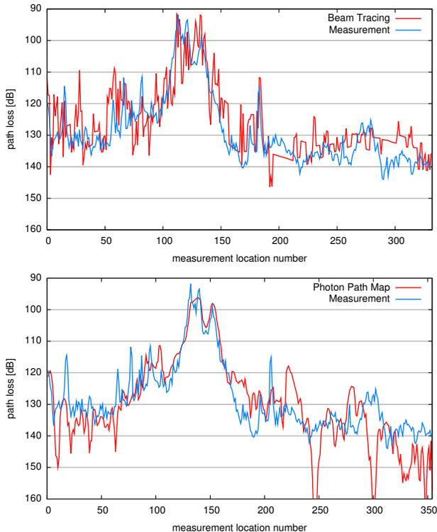
Fig. 3. Results of the prediction for the Munich route-1 scenario for the Beam Tracing (top) and Photon Path Map (bottom).
